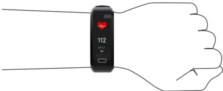
NOTE: The heart rate sensor is located on the back of the device. to monitor heart rate more accurately. Please wear the Nuband on the upper position of your wrist and a bit tighter than usual when you are doing exercise
