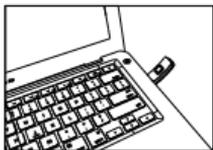
Tips: When charging, please make sure that screen side is facing down as shown in picture. If the charging does not respond, reverse the USB direction.
