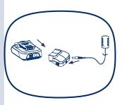
This product comes with a lithium ion battery pack. Lithium Ion batteries don't lose charge when not in use, and don't lose charging capacity overtime. Never the less it is best practice to charge the battery when empty or insufficient to do the job.
