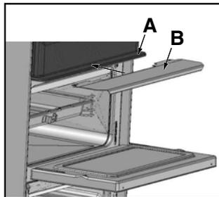
Slide the grill pan along the runner towards the rear of the grill compartment until it stops. An odour may be noticed when first using the grill - this should cease after a short period of use.
