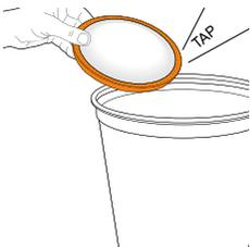
Tap the pre-motor filter against a bin to remove any dirt/debris.
