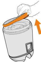
Lift out the pre-motor filter.
