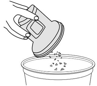
Tap the separator against a bin to remove any dirt/debris.
