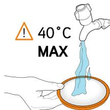
Rinse the pre-motor filter under water (max 40°C).
