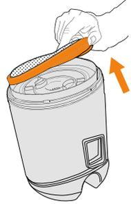
Lift out the pre-motor filter.
