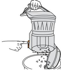
Hold the dirt container over a bin. Press the dirt release clip at the bottom of the container. The dirt release door will open allowing dirt/debris to fall out.
