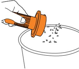
Tap the shroud against a bin to remove any dirt or debris. Using a dry cloth wipe the separator and shroud clean.
