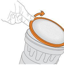
Lift out the pre-motor filter.
