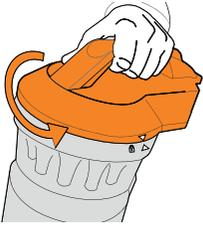
Twist the dirt container lid anti-clockwise and lift to remove.
