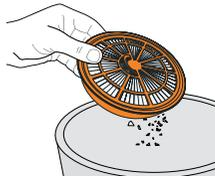
Check the post-motor filter for discoloration.
