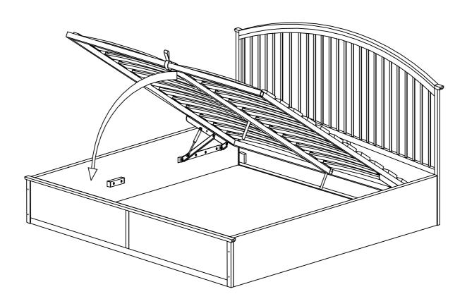
Lift with the strap (H12) and close as per guidance on page 8. The strap should always be accessible. Take care not to lean over the bed when lifting, if the mattress is thin and light, the frame may rise quickly. The speed of closing will also depend on the weight of the mattress so always keep fingers well clear of the metal frame.
