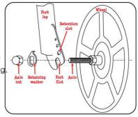
• Tighten both domed axle nuts securely with your spanner.
