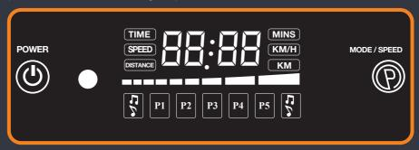
The readings scroll through Time, Speed and Distance. These show the time remaining of the programme you are on, the speed increment at which the machine is running, (between 0 and 99), and the equivalent distance you have walked/jogged/run.
