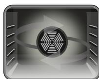
**Pizza Function:** The oven's thermostat and warning lights will switch on, and the ring, lower heating elements and fan will start operating. This function is ideal for baking food, such as pizza, evenly in
