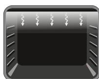
**Faster Grilling Function:** The oven's thermostat and warning lights will switch on, and the grill and upper heating elements will start operating. This function is used for faster grilling and for grilling food with a
