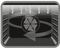
**Double Grill and Fan Function:** The oven's thermostat and warning lights will switch on, and the grill, upper heating elements and fan will start operating. This function is used for faster grilling of thicker food and
