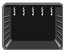
**Grilling Function:** The oven's thermostat and warning lights will switch on, and the grill heating element will start operating. This function is used for grilling and toasting foods on the upper shelves
