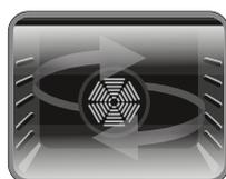
**Fan Function:** The oven's thermostat and warning lights will switch on, and the upper and lower heating elements and fan will start operating. This function is good for baking pastry. Cooking is carried out by the
