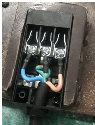
Fasten the wires beneath the screw heads
