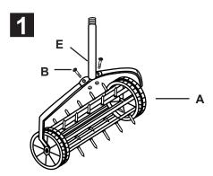
1. Using(B)part screw fittings screw the head(A)to the tube(E),please sure to righted all fixings securty.
