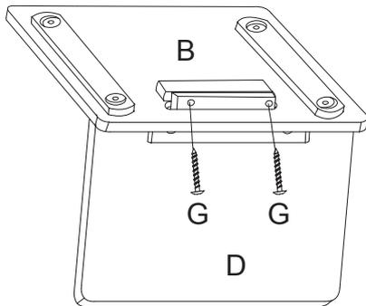
Secure Seat Back D to Seat B using 2 x Screw G.
