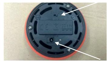
CHARGE PORT. Install USB cable here and connect to computer / output charger to charge.
