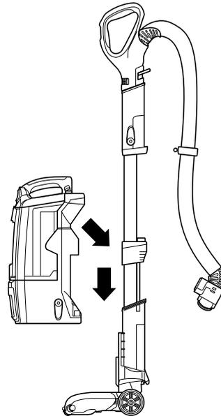
**3** Place pod onto wand and slide down to connect.
