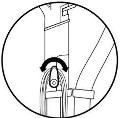
**TIP:** Use cord clip located on the side of wand to hold cord in place while vacuuming.
