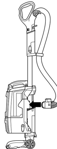
**4** Connect hose into back of pod, pressing it in until it clicks securely into place.
