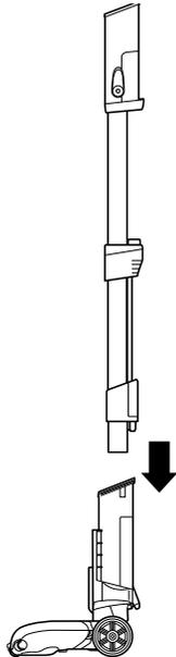
**1** Place motorised floor nozzle on floor and insert wand, pressing it in until it clicks securely into place.
