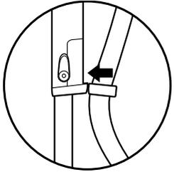
**TIP:** For quick cord access, rotate upper hook down and remove cord.
