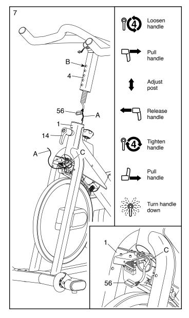
8. **See the inset drawing.** Connect the connector on the Upper Wire (56) to the connector on the Lower Wire (82).
