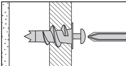
For use when attaching light loads on to plasterboard partitions.
