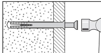
For use with walls stuck with plasterboard. The hammer fixing allows it to be fixed to the wall rather than the plasterboard. Always check the fixing is secure to the retaining wall.
