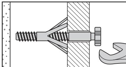
For use when fitting or supporting heavy loads such as shelving, wall cabinets and coat racks.
