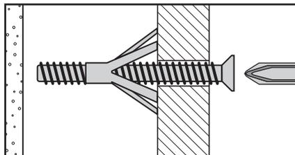
For use with plasterboard partitions or hollow wooden doors.
