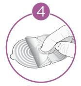
Remove clear protective film from gel pads, do not remove gel pads from device.
