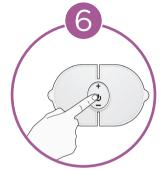
Press On/Off for 3 seconds to turn on the device.
