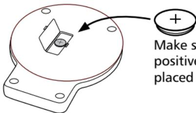
Make sure that the positive + side is placed upwards
