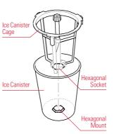
2 Insert the Ice Canister Cage into the Ice Canister. Make sure the Hexagonal Socket on the Ice Canister Cage aligns with the Hexagonal Mount in the Ice Canister.
