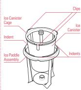
3 Insert the Ice Canister complete with Ice Canister Cage into the Ice Paddle Assembly so that the Clips line up with the 3 Indents. Make sure the Ice Canister is correctly seated. Carefully push each Clip into place. A loud 'click' will indicate each Clip is securely in position.
