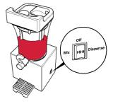
Note: If the Ice Canister jams, simply turn the machine off and wait for the ice to melt around the canister, enough to allow the blades to rotate again. Once this has melted enough, add ice again, slowly and regularly to cool the canister enough to make slush.
