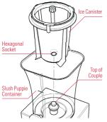
4 Insert the assembled Ice Canister into the Slush Puppie Container. Make sure the Hexagonal Socket on the Ice Canister aligns with the top of the Coupler in the Slush Puppie Container and slots firmly into place.
