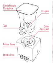
1 Insert the Slush Puppie Container onto the Motor Base. Make sure the Coupler on the Slush Puppie Container is correctly aligned with the Drive Sprocket and slots firmly into position. The Tap should sit directly above the Drinks Tray.
