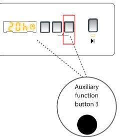
You can use this auxiliary function to delay the start time of the washing cycle for 1 to 23 hours .
