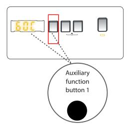
Use the washing water temperature adjustment button to alter the automatically programmed washing water temperature.
