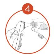
Use a new probe cover with each and every measurement – ensure probe cover is fitted on firmly before use.
