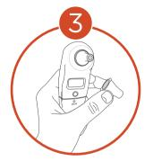
Remove protective cap covering probe lens.
