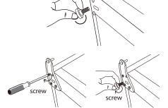
7. Reattach the bottom screws, bottom hinge and levelling feet to the opposite side of the unit bottom. Loosely secure.
