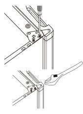
9. Put the top cover back and fix it in place with the screws.
