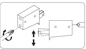
iii. When unit is hanging on the brackets, tighten lower screws clockwise, so clamping unit to wall - do not over-tighten.
