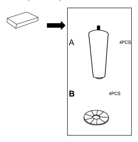
3. Fitting the legs on the bottom of the seat with correct orientation.
