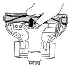
Rotate the brush to ensure free movement of the belt.
