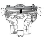
Remove brush assembly and check for wear on the belt.
