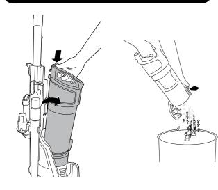
1 To remove the bin from the cleaner press the bin release button.
