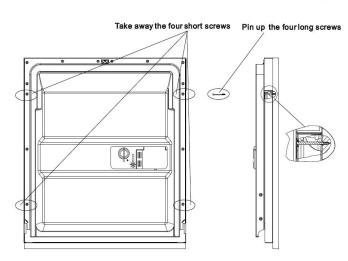
Figure 4B Installation of aesthetic wooden panel
