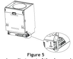
Tension adjustment of the door spring
