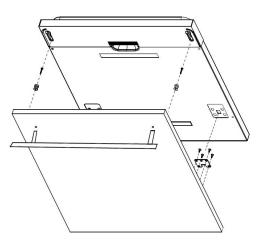
Figure 4A Installation of aesthetic panel
