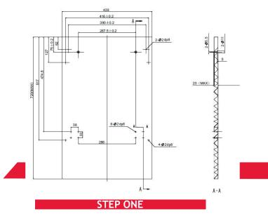
(Fig 3) The aesthetic panel should be processed in accordance with the illustrated dimensions (unit: mm)
