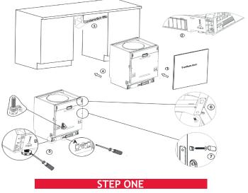
Install the furniture door to the outer door of the dishwasher using the brackets provided. Refer to the template for positioning of the brackets.
