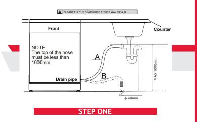
Insert the drain hose into a drain pipe with a minimum diameter of 40mm, or let it run into the sink, making sure to avoid bending or crimping it. The top of the hose must be less than 1000mm.
