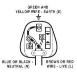
The BLUE wire must be connected to the terminal marked with the letter N
