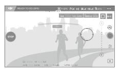
The aircraft will automatically adjust its speed when it senses an obstacle in front or if it is flying too close to the ground. However, this feature should not be relied upon for navigation between obstacles. Failsafe procedures will override TapFly. If the GPS signal weakens, the aircraft will exit autonomous flight and return to home.
