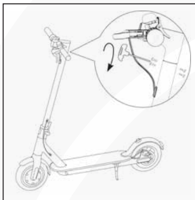
3. Using the allen key supplied tighten the screws to secure handlebars in stem.
