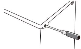
10. With the door closed, check that the door is aligned horizontally and vertically and that the seals are closed on all sides before finally tightening the bottom hinge. Re-adjust the levelling feet as needed.
