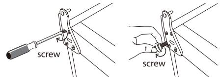
8. Carefully set the door back into place. Install the upper hinge and screws. Ensure the door is aligned horizontally and vertically so that the seals are closed on all sides before finally tightening the upper hinge. Use a spanner to tighten it if necessary.
