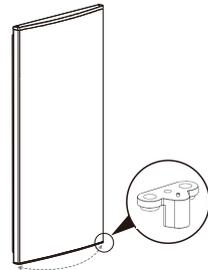
5. Remove the bottom screws, bottom hinge and levelling feet from the unit bottom.
