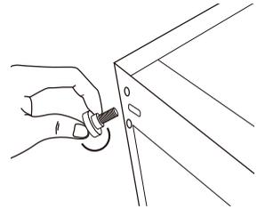
7. Reattach the bottom screws, bottom hinge and levelling feet to the opposite side of the unit bottom. Loosely secure.
