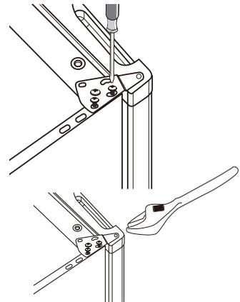
9. Put the top cover back and fix it in place with the screws.
