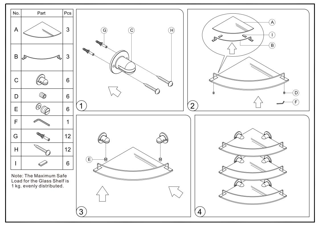
Wall Mounting: Hold the Fixing Template against the wall in the desired location and check if it is horizontal. Mark the wall to indicate where to drill the holes.
