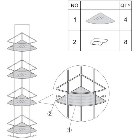
FOR MAXIMUM STABILITY, IT IS ADVISED THAT THE UNIT IS SECURED TO A WALL USING THE FIXINGS PROVIDED
