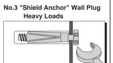
For use with heavier loads such as TV & HiFi Speakers and Satellite Dishes etc.
