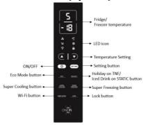
SETTING Button: Press "SETTING" to change the temperature.
