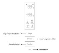
**TEMPERATURE SETTING:** Click the "Fridge" or "Freezer" button and when it flickers in the symbol, temperatures can be set. Each time when the button is clicked, the temperature changes accordingly. Temperatures cannot be set under functions of fast cooling, fast freezing, Smart ECO and vacation. Under temperature setting, if there is no button operation in 5 seconds, the button stops flickering and the set temperature comes into effect.
