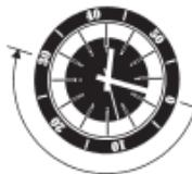
If your watch is equipped with a rotatable outer dial with one-minute graduations, this can be used in various ways to check elapsed time. For example if a diver has a 30-minute air supply, he can set the outer ring so that the triangle is in line with the minute hand when he submerges. The minute hand will then indicate on the outer ring the length of time that the diver has been under water.
