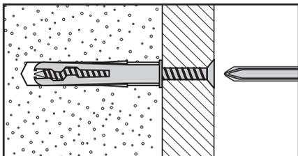
Generally aerated blocks should not be used to support heavy loads, use a specialist fitting in this case. For light loads, general purpose wall plugs can be used.
