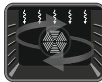
**Grill and Fan Function:** The oven's thermostat and warning lights will switch on, and the grill heating element and fan will start operating. This function is ideal for grilling thicker food. Use the upper shelves
