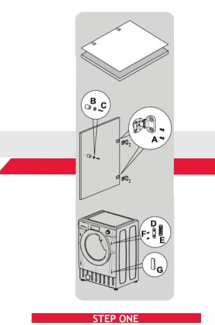
Position the template onto the reverse of the door. The hinges & closure magnet can be fitted on the right or left hand side depending on your requirements. Mark the screw holes positions, then drill out these positions.
