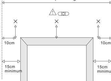
The end brackets must be positioned 10cm in from the end of the pole.
