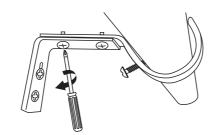
Loosen screws slightly, adjust to required extension, re-tighten screws.
