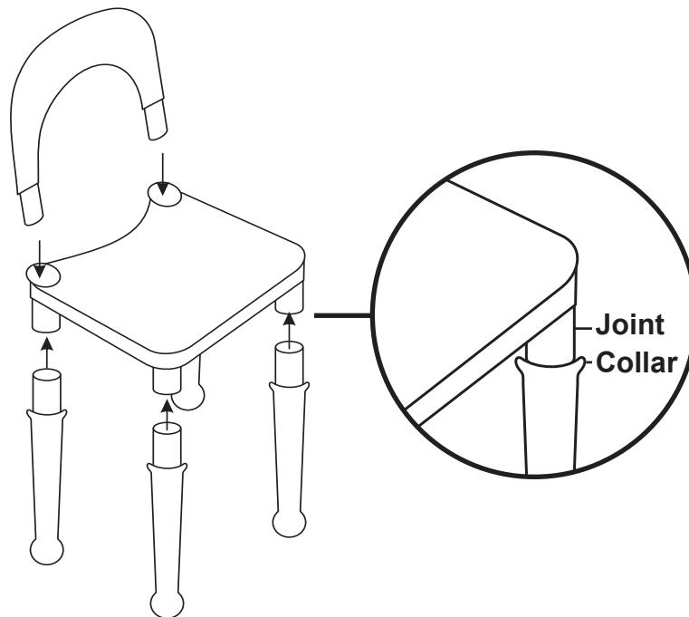
Push with force to ensure the legs are fixed properly. The leg collar should sit firmly against the joint.
