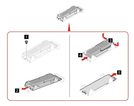
Note: Remove the film that covers the thermal pad (if any) when installing the M.2 solid-state drive and heatsink.
