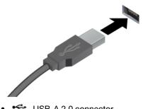
Connect USB-A compatible devices, such as a USB-A keyboard, USB-A mouse, USB-A storage device, or USB-A printer.
