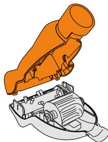
Replace the bottom cover, insert and tighten the screws.
