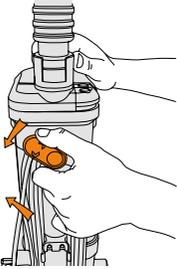
Twist the quick release cord hook to release the power cord.
