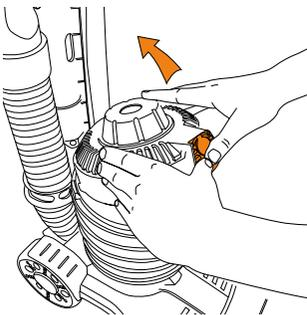
Press the button on the post-motor filter cover and remove.
