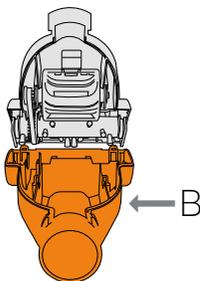
Remove the bottom cover (B). Clean out any debris or hair from the brushbar and turbine fan.
