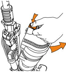
Press the dirt container release button and pull to remove the dirt container.
