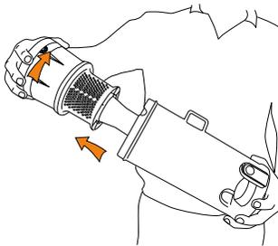
Lift to remove the separator from the dirt container
