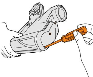
Using a crosshead screwdriver, remove the 3 screws from the belt cover on the side of the floorhead.
