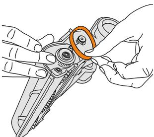
Clean any debris from the cogs. To replace the belt firstly hook the belt over the small cog. Slide the belt over the top of the large cog and rotate the belt and cog anticlockwise. During rotation the grooved belt will slide onto the cog.
