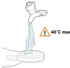
Wash the filter under running water (40°C max).
