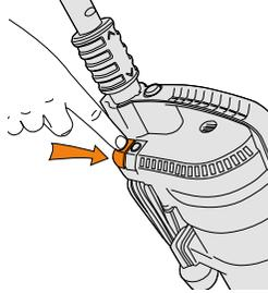
Plug in your machine and push ON/OFF button to switch on.
