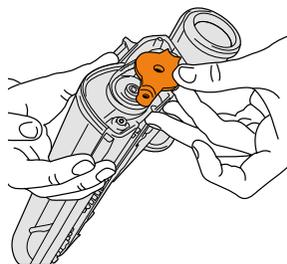
Pull to remove the brushbar location plate and remove the belt. If the belt isn't broken rotate the cogs anticlockwise and slide the belt off the large cog first.
