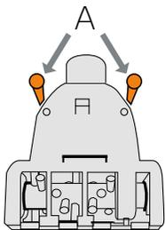
Clean the TurboTool by removing the 2 screws (A), located on the bottom cover, with a crosshead screwdriver.
