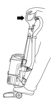
1 Plug power cord into outlet. Place foot on floor nozzle and tilt handle back.
