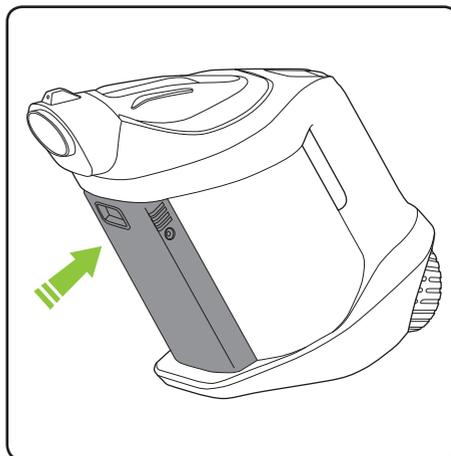
Push the battery into the slot until it clicks into place. If you want to buy a spare battery go to [www.gtech.co.uk](http://www.gtech.co.uk) or call **01905 345891**.
