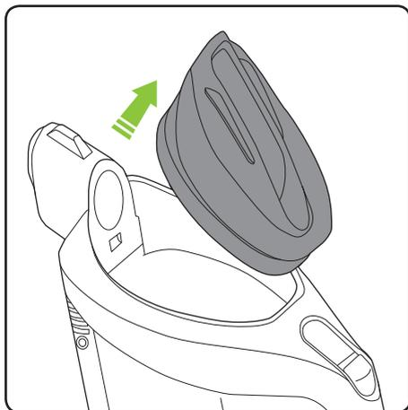
Remove the lid by pulling gently upwards.
