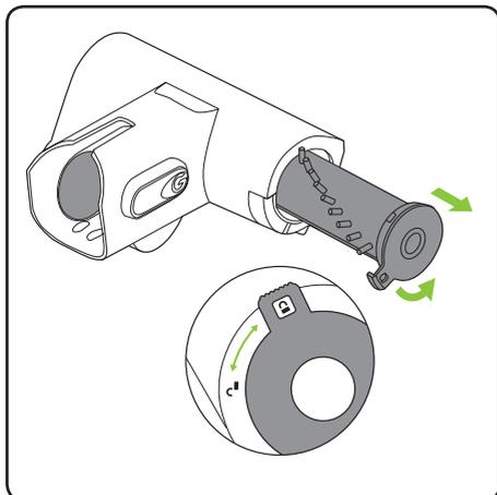
To clean the brush bar, first remove the power brush from the Gtech Pro. Rotate the latch from the lock to the unlock position and pull out to remove the brush bar.
