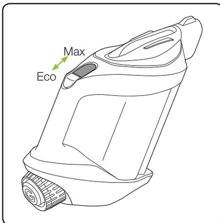
The GtechPro has 2 power settings: Max mode (higher suction power and shorter runtime) and Eco mode (lower suction power and longer runtime). Change modes by sliding the switch located in front of the on/off button. The Gtech Pro will turn on in the mode it was last used.
