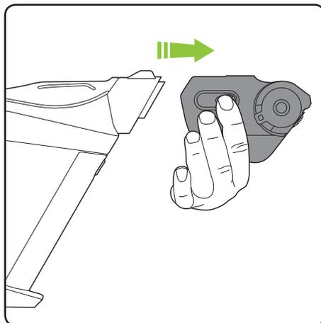
To remove the power brush, press the latches on the sides of the power brush and pull it away from the main unit.
