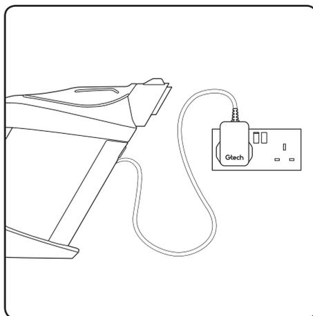
Plug the charger in and connect it to the charging port at the side of the battery.
