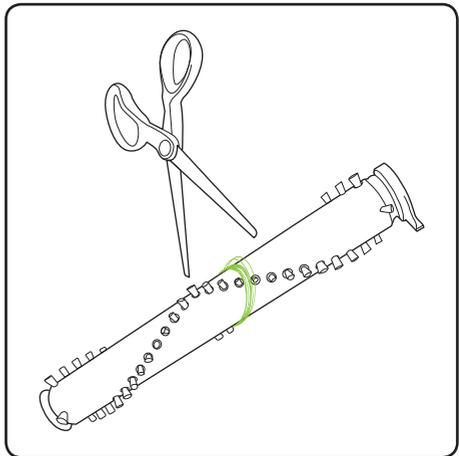
To remove hair from the brush bar, run an open pair of scissors down the groove to cut the hair, then pull it out. Never operate the power floor head without the brush bar in.
