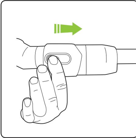
To remove the extension tube and floor head, press the buttons on the sides of the attachments and pull it away from the unit.
