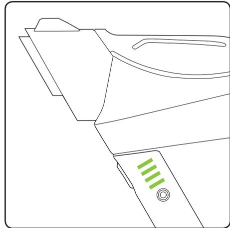
While the battery is on charge, the LEDs will pulsate and in turn illuminate. When the battery is fully charged all of the LEDs will be solid green.
