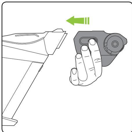
To attach the power brush line up and slot it over the Gtech Pro nozzle. The power must be off when changing accessories. (The power button will now activate the power brush as well as the suction.)
