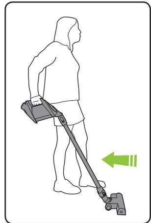
Pulling the vacuum back towards you activates the AirLOC and picks up fine particles.
