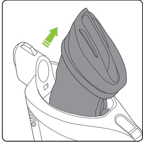
When the bag is full, lift the lid and remove from the Gtech Pro with bag attached.
