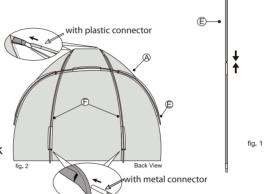
5. Bend the Black Fibreglass Poles © so that the ends fit into the rings in the corners of the Shelter A.
