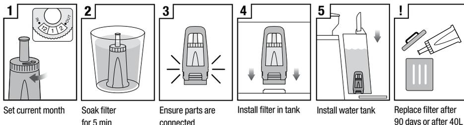
The provided water filter helps reduce the risk of scale build-up in and on many of the inner functioning components. Replacing the water filter after three months or 40L will reduce the need to descale the machine.
