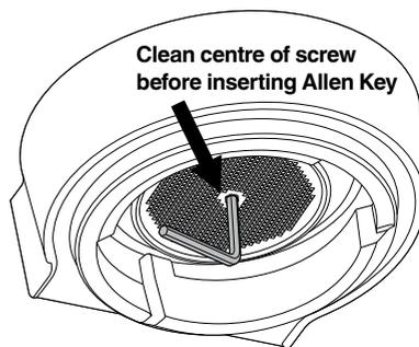
5. Once loosened, carefully remove and retain the screw and stainless steel shower screen. Make note of the side of the shower screen that is facing downwards. This will make re-assembly easier. Wash the shower screen in warm soapy water, then dry thoroughly.
