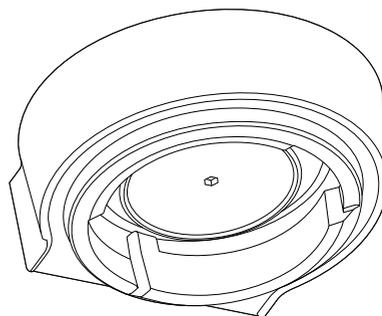
7. Re-insert the shower screen, then the screw. With your fingers, turn the screw clockwise for 2-3 revolutions then insert the Allen Key to tighten until the screw is flush with the shower screen.
