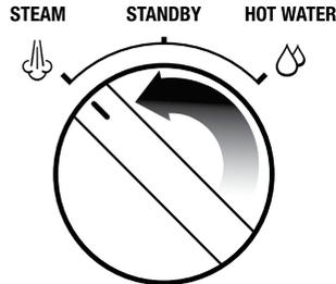
3. Rotate the STEAM/HOT WATER dial to the HOT WATER position and run water through the hot water outlet for 10 seconds.
