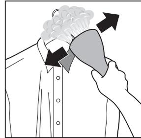
**EN** Keep the steamer head a slight distance away from dresses with frills, ruffles, ruching or sequins. Use only the steam to loosen the fabric. You can also steam from the inside.
