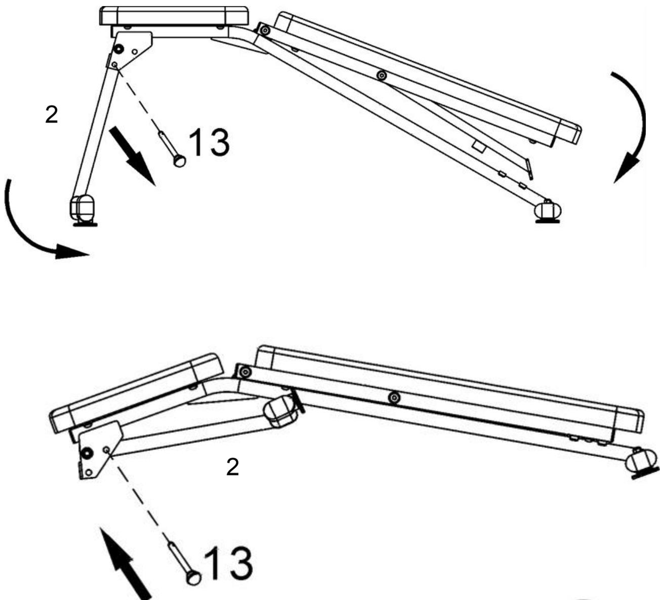
Remove the Lock pin(13),folding the Front Support(2) and the Backrest, then insert the Lock Pin(13) into the lock position as shown in the diagram.
