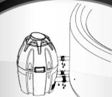
Check and ensure the Spa and adapters are not leaking.
