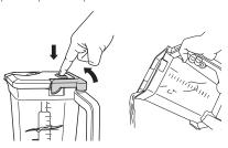
8b For thicker mixtures that cannot be emptied through the pour spout, remove the lid and Stacked Blade Assembly before pouring. To remove the lid, press the RELEASE button and lift the handle. To remove the blade assembly, carefully grasp it by the top of the shaft and pull straight up. The Jug can then be emptied.
