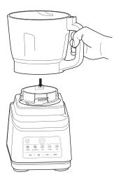
**2** Lower the Food Processor Bowl onto the motor base and rotate clockwise until it clicks into place.
