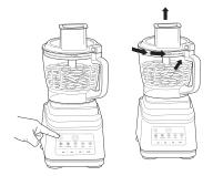
8 When finished, stop the unit by touching the Power button and wait for the disc to stop spinning. Press the button on the feed chute lid near the handle to unlock, then turn the lid anticlockwise. Lift the lid from the bowl.
